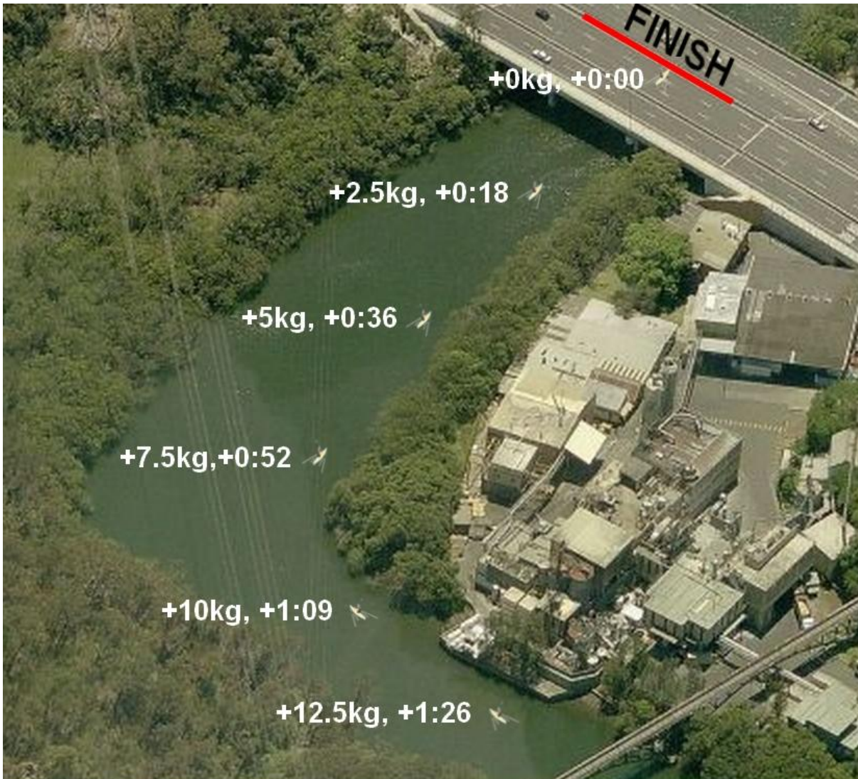
Figure 2: Effect of extra dead weight on average paddler's 12km finishing time (65 minute 90kg paddler)
