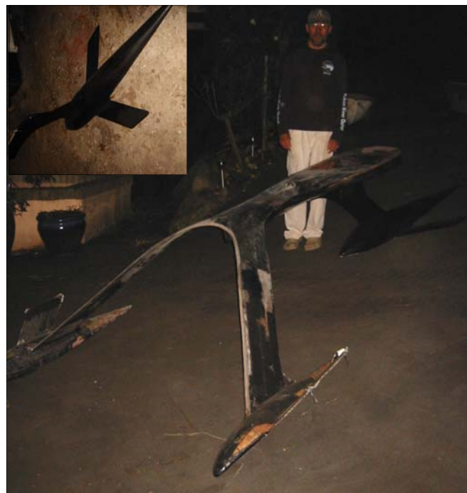
The front of the subrofoil has two forward submarines (like torpedoes), with hydrofoils which are angled up on the outside for directional and rough-water stability. Under the seat at the rear is the central submarine, with horizontal hydrofoils. The submarines are made from hollowed-out foam covered with carbon-fibre which gives buoyancy. The 1.5m-long seat is like a waveski seat. The craft is about 4m long, 0.8m high and 1.5m wide at the front submarines. When stationary, only the top is out of the water. In motion, the top will be about 20cm out of the water. Any higher would be hard for paddling. Inset: The main submarine of the subrofoil with its horizontal hydrofoils and the vertical extension to the seat.
