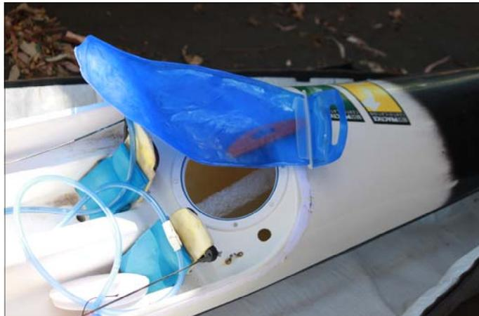
I added a windscreen-cum-cowl over my legs at the front of the cockpit. This kept water out of the foot well and offered a bit of streamlining for upwind work. The screen was simply velcroed on. This arrangement made the boat sort of a hybrid kayak/ski and Apollocraft will offer it as an optional extra. The screen gave me a mounting position for my GPS in a position so it was just in my field of vision.
