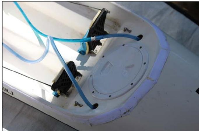
This padding also moved my seating position forward about 100mm, so I was able to take out the adjustable foot pedals and mounted the pedals
