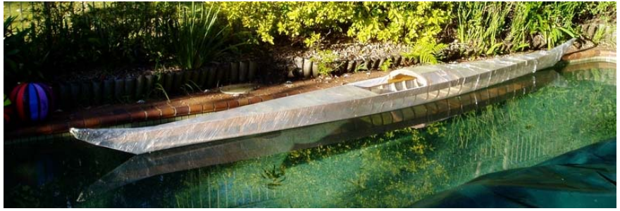
Wrapped in clear plastic, the kayak is tested in a swimming pool. Rob paddled many times in the see-through, shrink-wrapped kayak in Lane Cove River.
