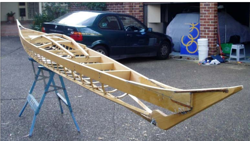
Hoop pine was used for the longitudinals and huon pine for the ribs
